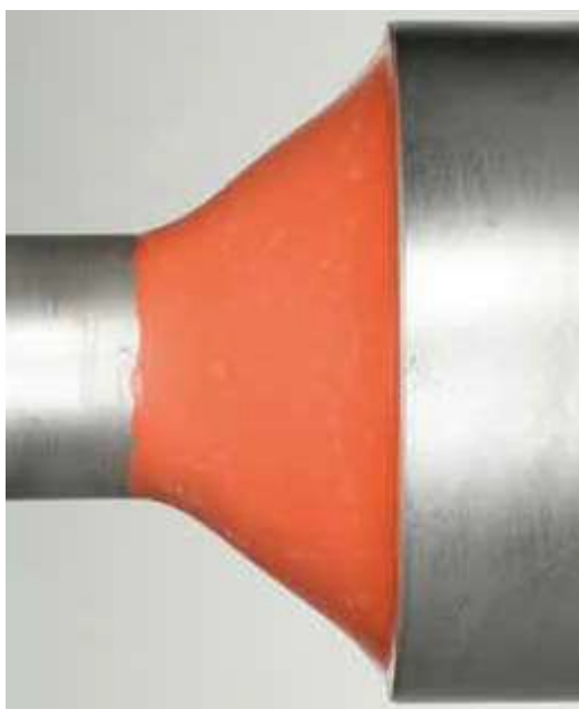
Figure 2. Displacement of the pipe in the longitudinal direction in relation to the outer transit wall with half of the diameter difference between the pipe and the transit wall.
